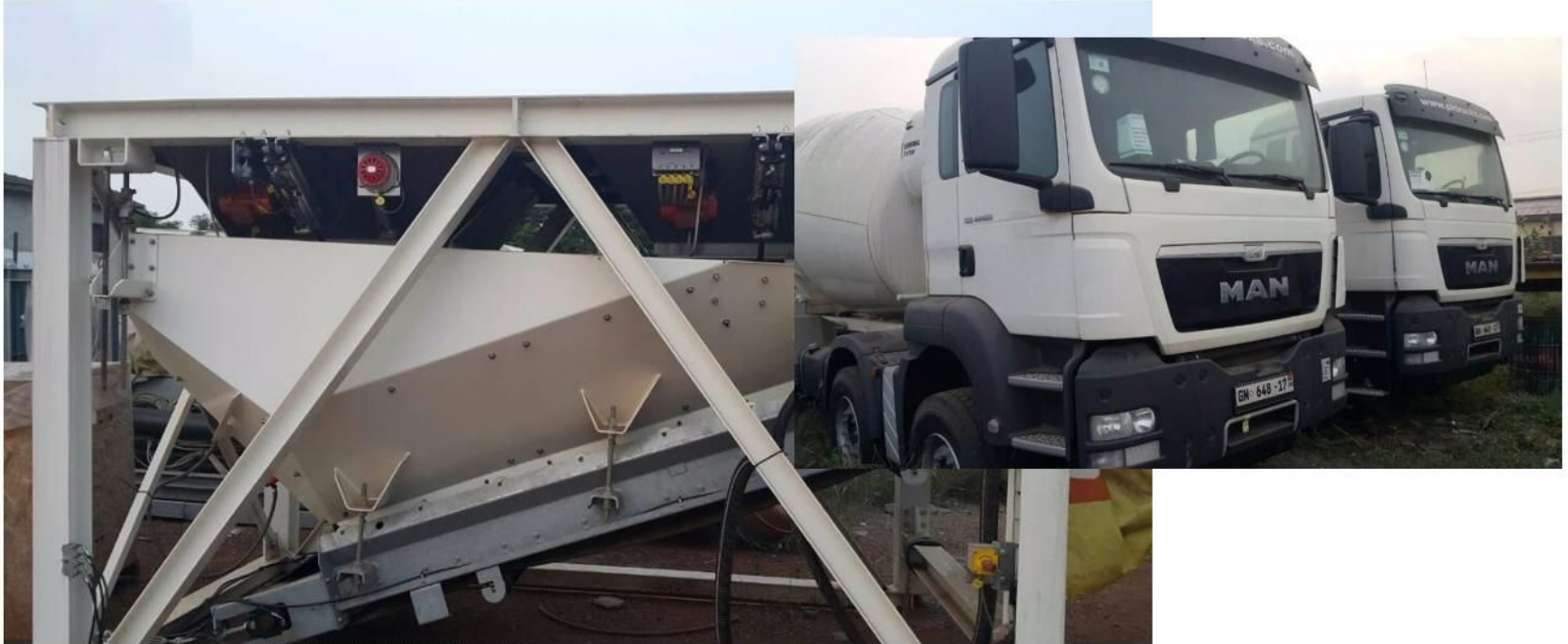
Concrete batching and handling equipment
